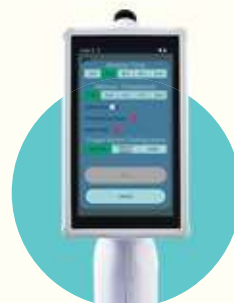
User adjustable settings for time and temperature of treatment cycle
